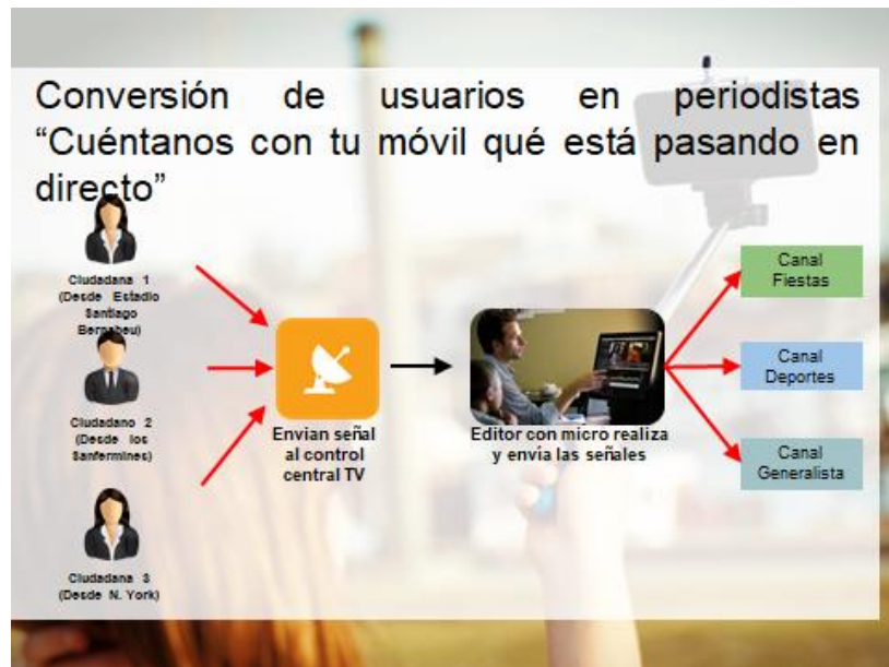
Figure 4. The process of sending the signal from the app to the central TV control where the signal is distributed to different channels
