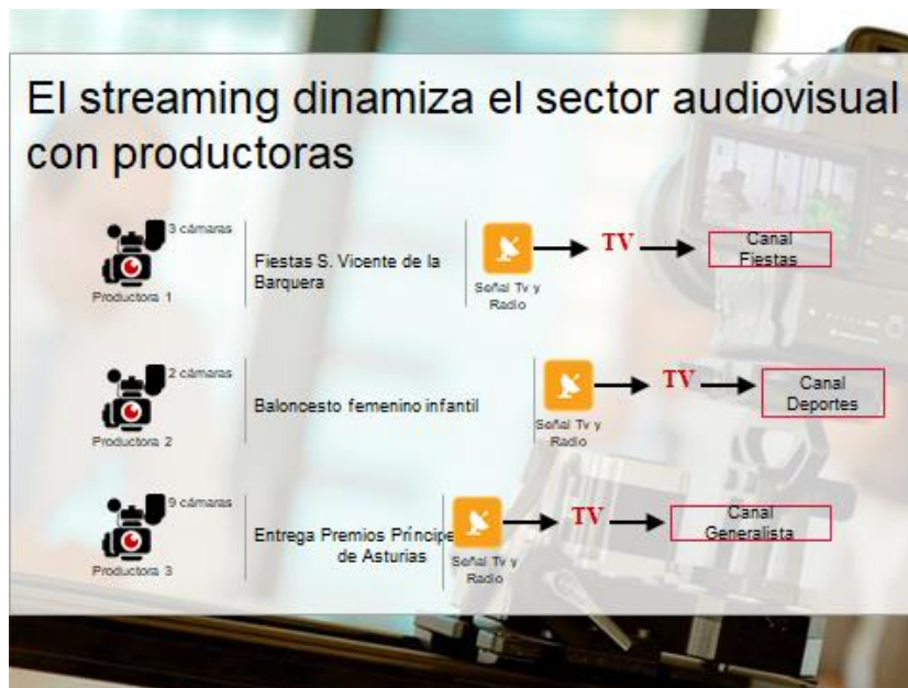
Figure 6. The process of sending the signal by streaming to the central TV control where the signal is distributed to different channels
